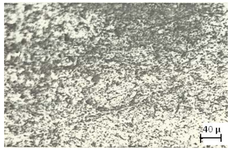
Fig. 9. Rapidly Solidified Al-7wt% Si, annealing at 500°C for 1hr, 500X.
